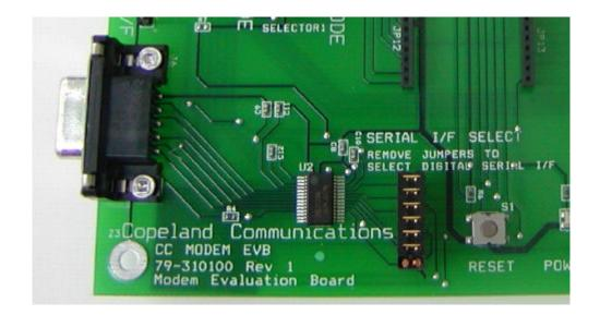
*¬RTS* - pin 33 – must be held high during reset (a 10K resistor or directly pulled to VCC) *SDI* - pin 40 – 10K resistor to VCC *¬FSYNC* - pin 24 – 10K resistor to VCC *SDO* - pin 27 – 10K resistor to VCC
