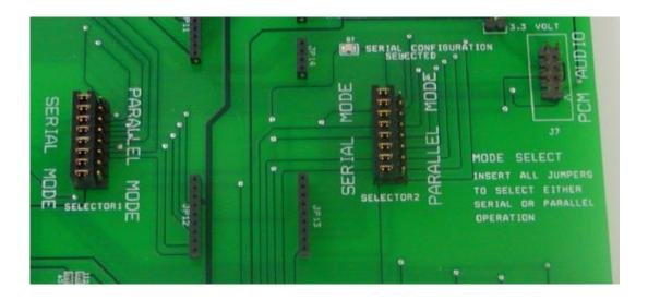
**SERIAL MODE INDICATOR** (D7) will light when both jumpers are in the serial mode position.
